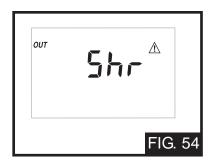
The control is no longer able to read the outdoor sensor due to a short circuit (FIG. 54). In this case the controlassumes an outdoor temperature of 32°F (0°C) and continues operation. Locate and repair the problem as described in INS7141. To clear the error message from the control after the sensor has been repaired, press either the Menu or Item button. This error message only occurs if the External Input / Stand Alone DIP switch is set to Stand Alone.
